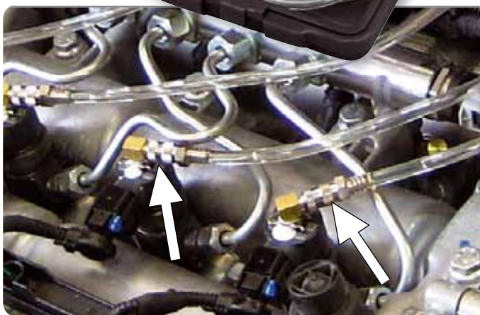
Quick Coupler Adaptor System - "No leak" connections.
