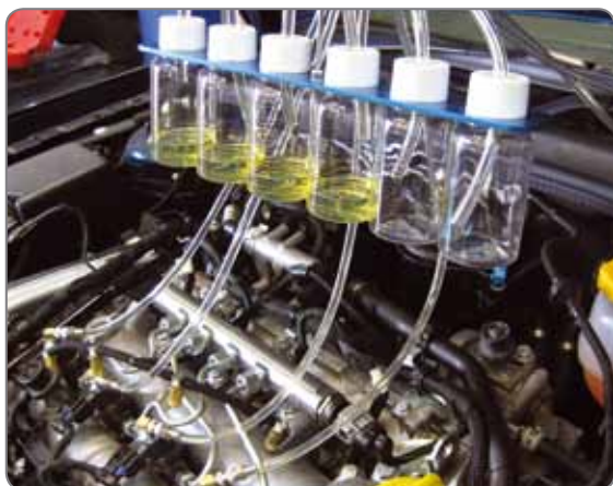
Fuel Measurement Hanging Rack Assembly.
